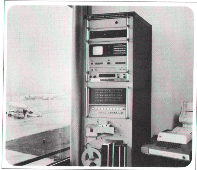
Fig. 4. The central processor can scan each noise monitoring terminal once each second, process the data, and present the results in the optimal form for evaluation by relatively untrained personnel. It can be adapted to future regulations and noise evaluation methods simply by changing programs.
