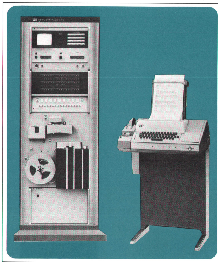
Fig. 1. Model 80501A Audio Data Processor consists of a real-time audio spectrum analyzer (with CRT) which measures the frequency spectra of audio-frequency inputs, a digital computer which processes the measured spectra, and peripheral devices. A typical application is aircraft noise analysis and evaluation. Real-time processing gives results almost immediately so appropriate action can be taken if required.
